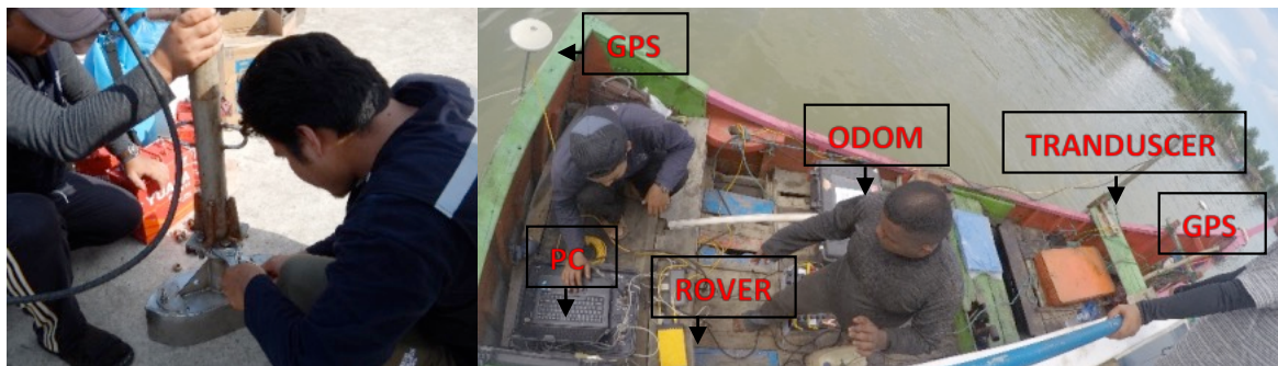
Figure 2. Transducer set-up and deployment using field survey
